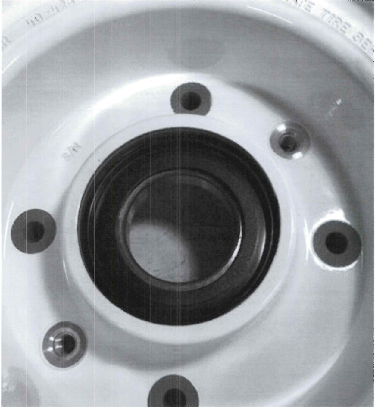
Figure 4 – Improper Grease Seal Orientation
