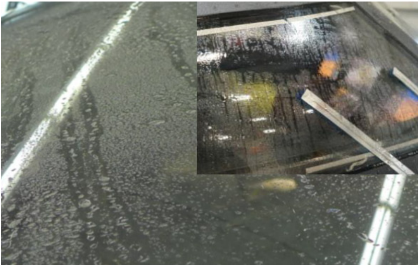
Figure 2-6-3: Windshields - Rain repellent (unsatisfactory condition)
