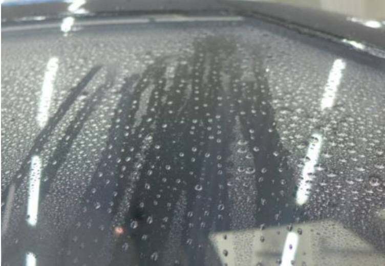
Figure 2-6-2: Windshields - Rain repellent (satisfactory condition)
