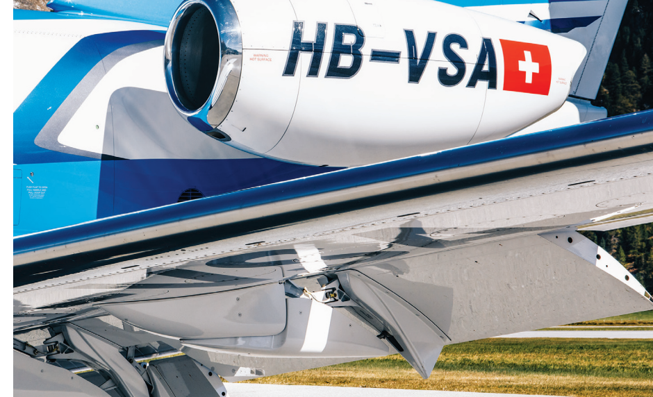
Double-slotted flaps and high-mounted engines prevent FOD contamination.
