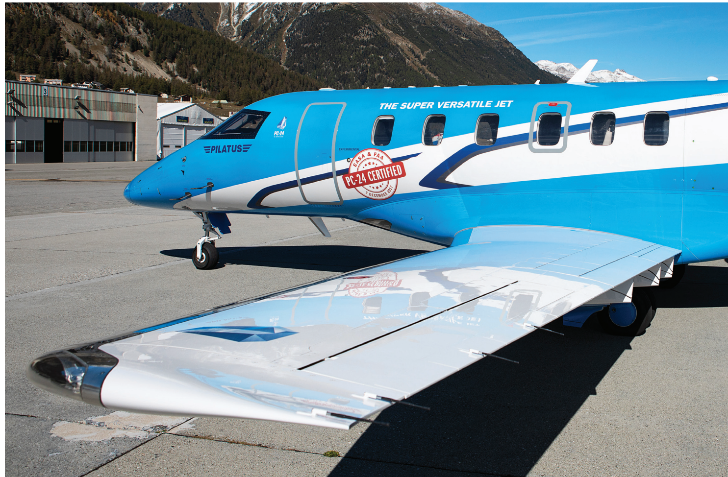
Low-pressure tires allow the PC-24 to land on unpaved runway surfaces.
