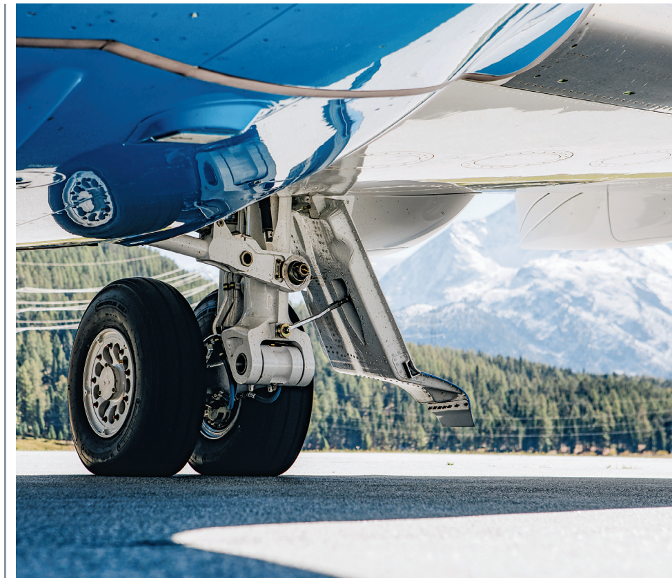
Low-pressure tires allow the PC-24 to land on unpaved runway surfaces.
