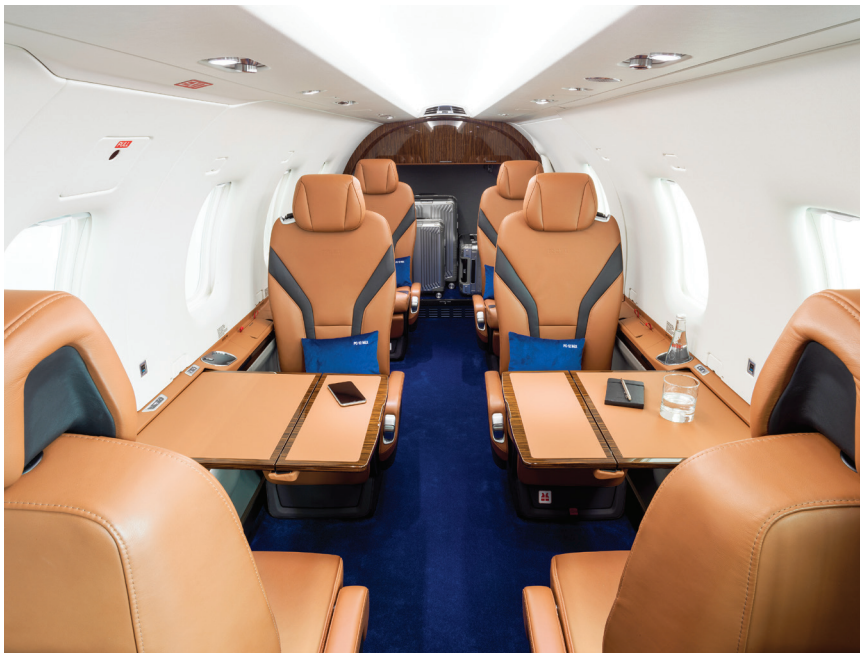
The 6 + 2 seat exterior interior is a $455,000 option. New chairs recline fully to create lie-flat berths. Quick release chair mounts allow interior to be reconfigured for cargo in less than 10 minutes. (Rearmost +2 seats not shown.)
