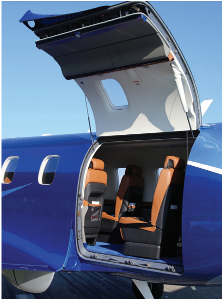
(Left) 18+ sq. ft. cargo door and flat cabin floor are favorite features with operators. (Middle) Full-cabin-width forward lav has flush toilet and full height privacy doors. (Right) New windows with squarer corners are 10% larger, flooding the cabin with considerably more ambient light.
