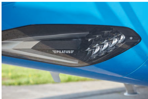
All interior and exterior lights, including the landing light arrays, use long-life LEDs.
