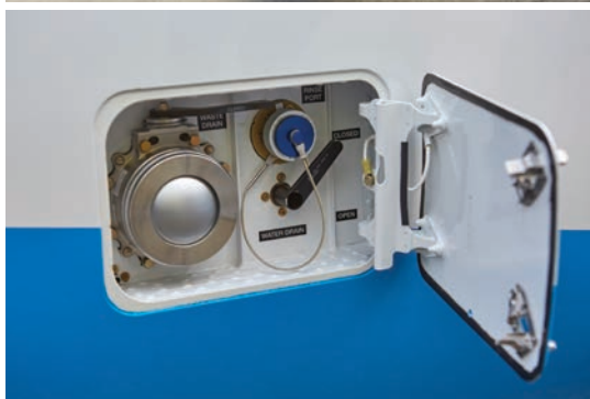
Top/Bottom: The single-point pressure refueling receptacle has selectable refill quantity pre-set feature. The PC-24 is the first midsize jet to have an externally serviced vacuum lavatory system.
