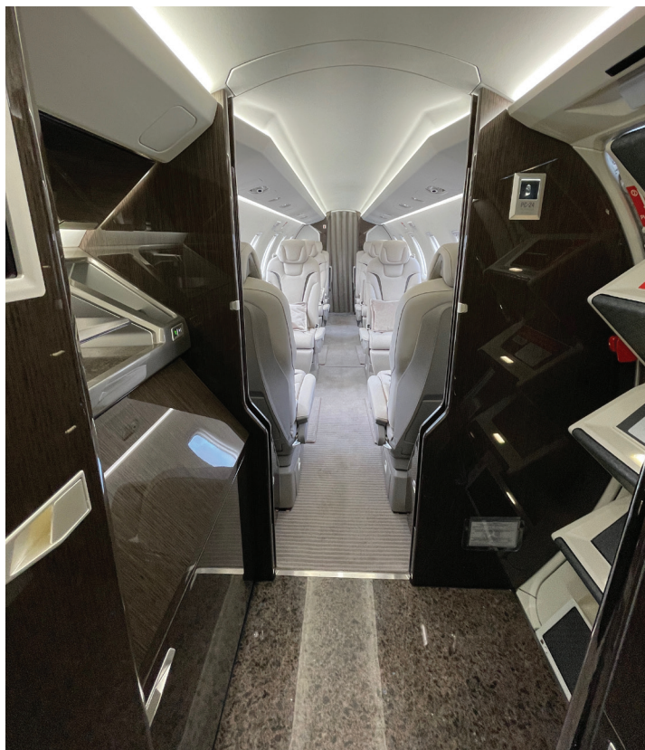
The PC-24's forward galley allows for maximum flexibility in cabin configuration and easy inflight access to the large cargo compartment.
