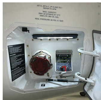
Single-point refueling is the quickest way to fill the PC-24 with a maximum load of 5,964 pounds of jet-A.
