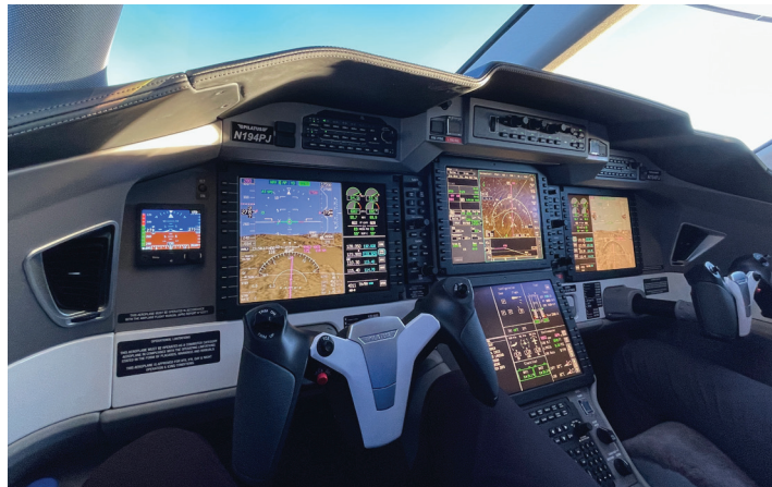
The PC-24 flight deck features a Honeywell Epic-based avionics suite, cursor-control device interface, and autothrottles.
